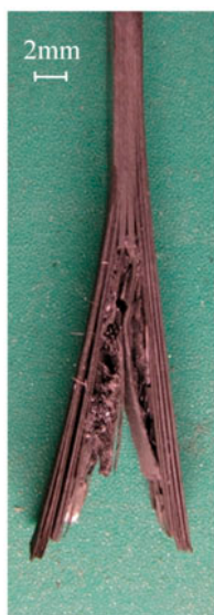
Figure 8. A unidirectionally laminated CFRP plate taken from the test fixture after progressive crushing test ( L_g = 15 mm).
